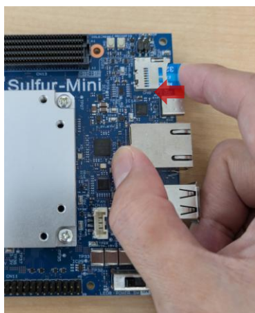
(a) Inserting the microSD Card
