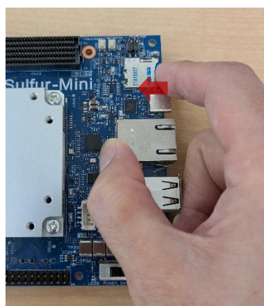
(b) Removing the microSD Card
